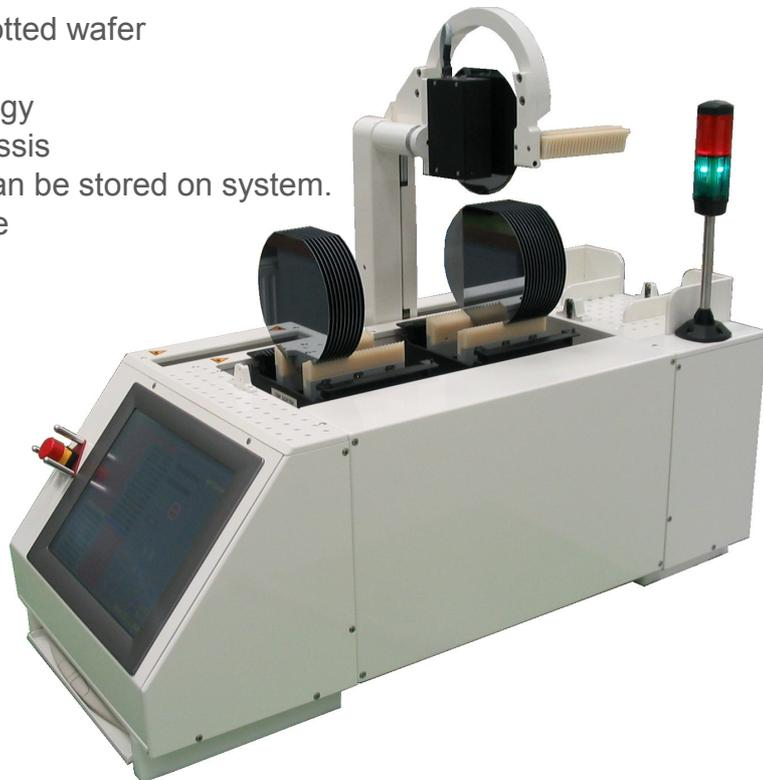
These models are compatible with most standard 4", 5", 6" and 8" plastic wet/dry process cassettes, shipping and storage containers.
