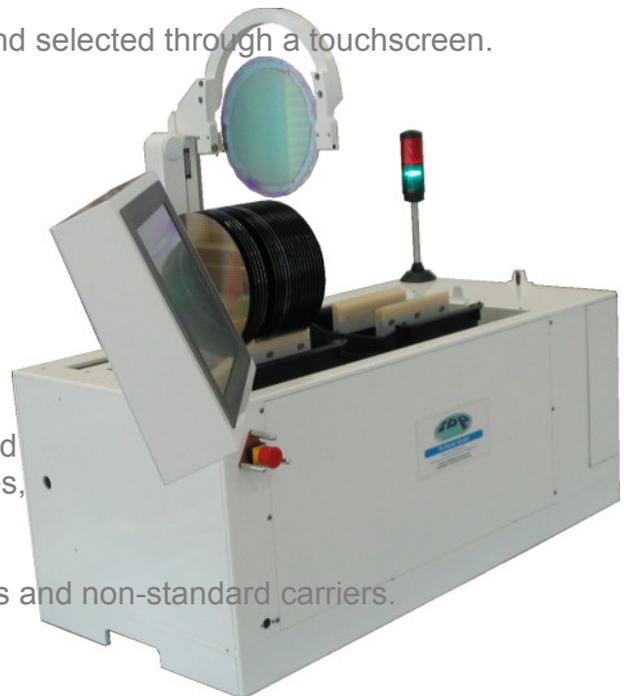
These models are compatible with most standard 4", 5", 6" and 8" plastic wet/dry process cassettes, shipping and storage containers.
